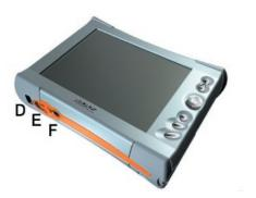
**D. USB 2.0 port** Insert USB cable mini jack here and attach other end to computer USB port. (USB 1.1 compatible).
